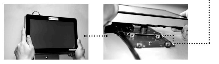
It is highly recommended that you screw in the **Wallmount Security Screws (N)** into the security extensions to mitigate the chance of theft or damage. From below your **WandaNEXT**, insert **N** into the threads of **K**s security ex-tensions and tighten with Philips Screwdriver until secure.
