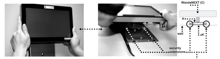
Allow the **WandaNEXT** to slide down until the security extensions from **H** rests on top of the security extensions from **K**. Make sure the slots from **H** are definitely hooked into the grooves of **K**, on both sides, to ensure that the **WandaNEXT** is fixed in place and doesn't fall when you let go.
