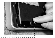
Once removed, insert the Phillips Screwdirver head into the newly exposed hole and proceed to remove **Detachable Back Cover Screws (B).**
