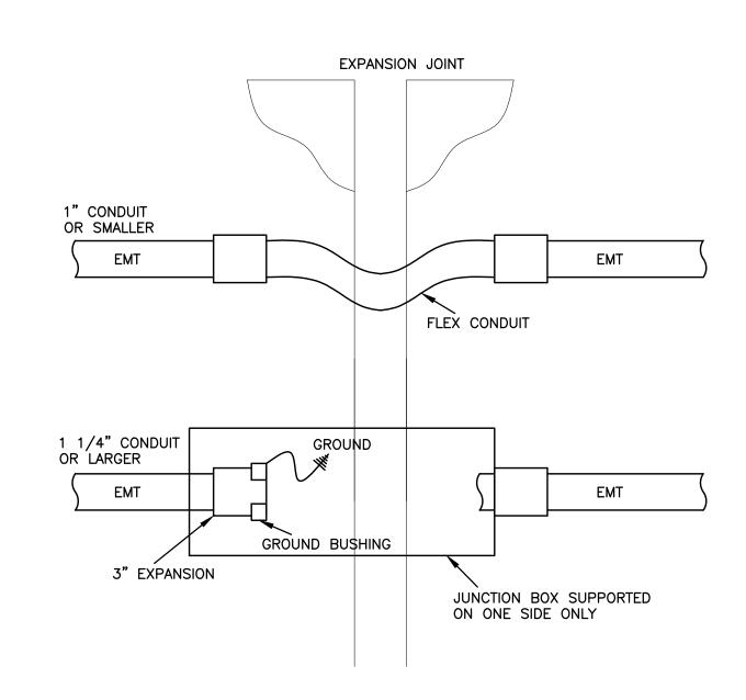
EXPANSION JOINT CROSSING DETAIL E-1.1 SCALE: NTS
